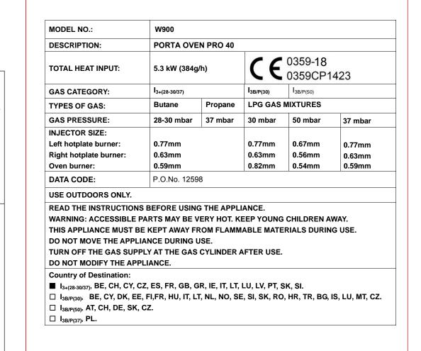
If there is strong smell when using the appliance, please turn off the gas supply and turn off the fire at once, also open the glass window!  Must use the appliance with country pressure standard and safety standard's qualified regulator and hose, it is very dangerous for using the unqualified regulator and hose.
